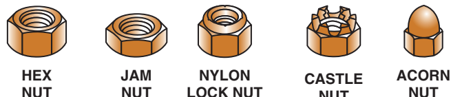
FIGURE 1-13 Nuts come in a variety of styles, including locking (prevailing torque) types, such as the distorted thread and nylon insert type.
