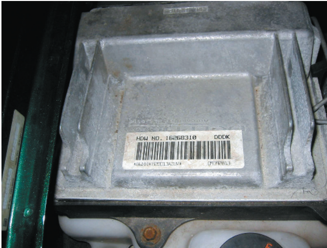
FIGURE 1-3 A typical calibration code sticker on the case of a controller. The information on the sticker is often required when ordering parts or a replacement controller.
