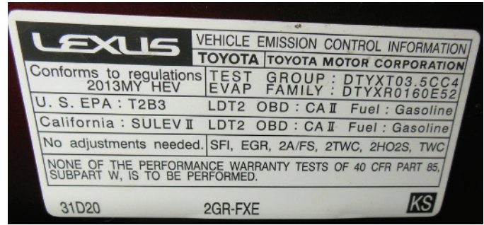
FIGURE 1-2 The vehicle emissions control information (VECI) sticker is placed under the hood.
