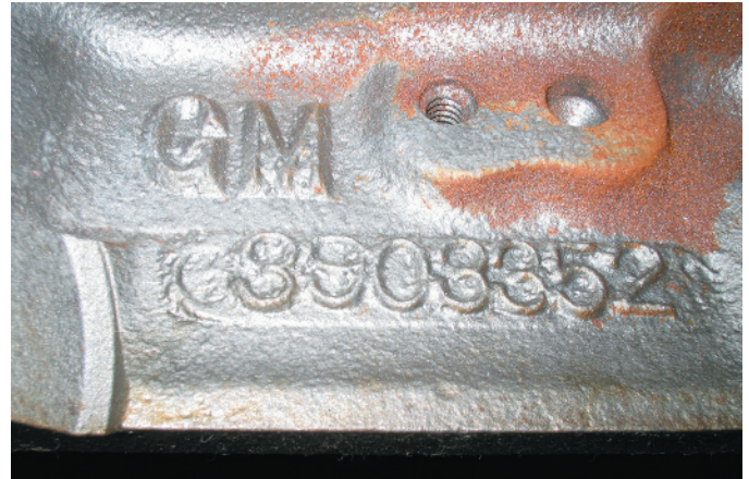
FIGURE 1-4 Casting numbers on major components can be either cast or stamped.
